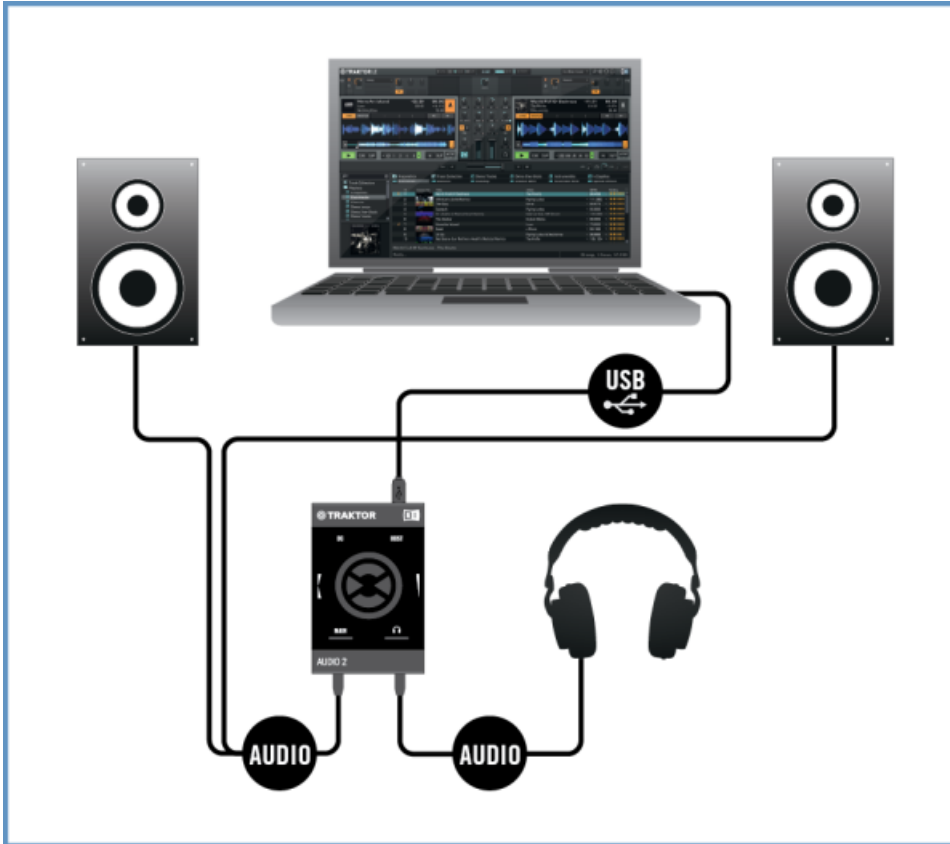
Setup overview of using TA2 in Internal Mixer Mode with a computer.
